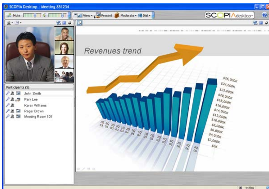
Figure 2: SCOPIA Desktop user interface H.239 data collaboration in the main window and simultaneous continuous presence H.264 video.
